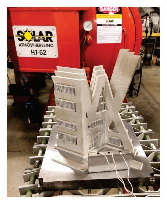
**Fig. 2** — Placing an external dummy block containing a thermocouple near the additively manufactured part provides a good comparative temperature profile for the part.
