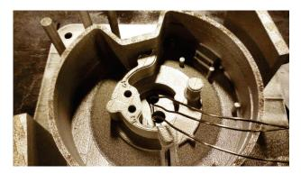
**Fig. 1** — Placement of a thermocouple in a hole in an additively manufactured part provides the most accurate temperature profile during heat treatment.
