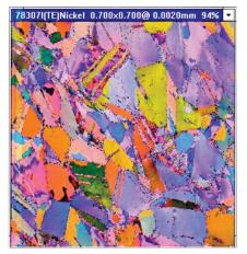
**Fig. 4** — Photomicrograph of nickel-base superalloy Waspaloy. This orientation imaging micrograph (electron backscatter diffraction pattern image) shows clear straining and polygonization within the deformed grains. Dark spots near grain and prior twin boundaries are a result of high localized strain and crystal orientation unable to be determined.
