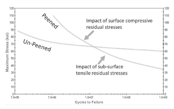
**Fig. 7** — Schematic of fatigue behavior of peened and nonpeened material for a specific nominal R-ratio. Peening shows clear ability to improve LCF capabilities over nonpeened, but as stresses are lowered the HCF life of peened material can show a debit over nonpeened due to interactions of applied and internal tensile residual stresses.
