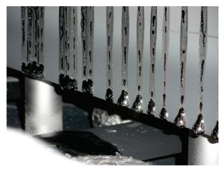
**Fig. 4** — Damage to a graphite-metal fixture from eutectic melting enabled by deterioration of old or reused silica textiles used to separate the graphite and metal.
