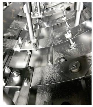
**Fig. 3** — Damage to vacuum-furnace hot-zone components due to harmful reactions of loose powder hidden in blind holes of the build plate blown throughout the furnace during the vacuum evacuation.
