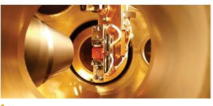
A sample of tungsten ditelluride in an ultrahigh vacuum chamber. Courtesy of AG Bauer.
