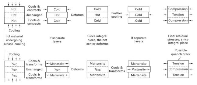
**Fig. 1** — Mechanisms of generation of bulk residual stresses. Top row depicts steps in the process of thermally induced residual stress formation; bottom row depicts steps in the process for phase transformation-induced residual stress formation<sup>[1]</sup>.
