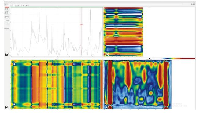
Fig. 4 — MW data image of wind turbine mock-up sample: Frequency and time related responses shown in A, B and C scan format.
