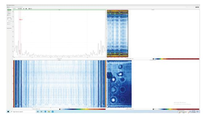
Fig. 7 — HDPE flat plate (24 x 12 x 1 in., inspected in 8 minutes) demonstrating location and sizing of multiple defects using advanced MW technologies now in development.
