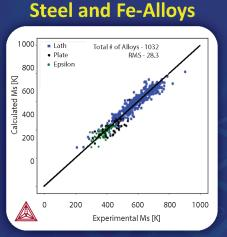
Comparison of calculated and experimental Ms temperatures for a wide range of steels
