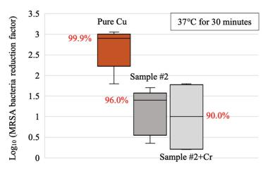
**Fig. 2** — Log<sub>10</sub> (reduction factor) of MRSA bacteria remaining after 30 minutes exposure at 37°C to pure Cu and two polished steel samples, one with 2.5 wt% Cu (sample #2) and the other, sample #2 with 12 wt% Cr added (sample #2+Cr), both after heat treatment to form nanometer-size copper precipitates. Median reduction percentage is noted next to each box.
