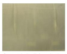
**Fig. 3** — Wind turbine blade sample with marcelling.
