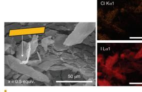
Left: Scanning electron microscope image of film fragments. Right: Elemental mapping indicates creation of hybrid perovskites. Courtesy of MIT.
