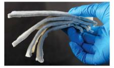
A sample of Empa's electromagnetic shielding material—a composite of cellulose nanofibers and silver nanowires.
