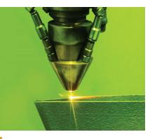
In 3D printed metallic parts, Argonne scientists found a correlation between temperatures at the surface and defects that form below.
