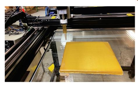
Fig. 1 — Microwave examination of Kevlar panel.
