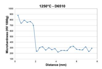
**Fig. 3** — Hardness profile of laser heat treated D6510 across the depth. Average hardness of 760 HV (62.5 HRC) was recorded on the D6510 test sample shown in Fig. 2.
