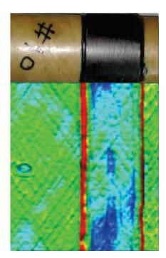
**Fig. 2** — Microwave inspection of highdensity polyethylene.
