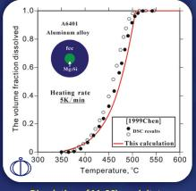
Dissolution of Mg2Si precipitate in Alloy A6401
