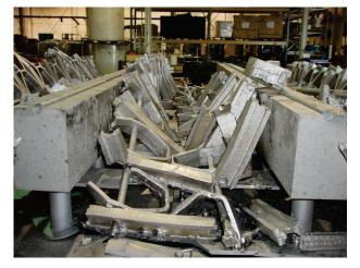
**Fig. 5** — Damage in the area of an Inconel alloy grid from eutectic melting due to exceedance of the eutectic temperature during furnace bake-out.
