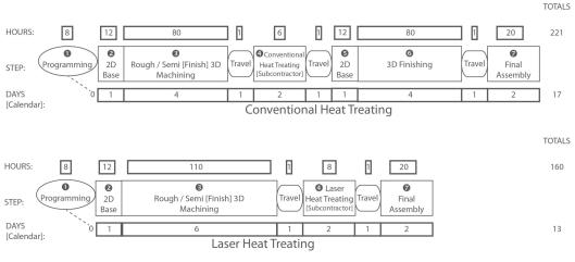
Fig. 5 — Set up of a conventional heat treating line, top, compared to a laser heat treating line, bottom.
