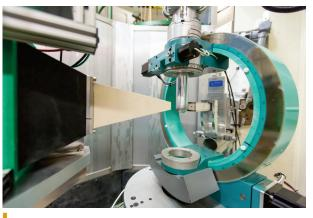
Researchers performed single-crystal neutron diffraction using the HB-3A four circle diffractometer to confirm the first intrinsic ferromagnetic topological insulator. Courtesy of Genevieve Martin/ORNL.
