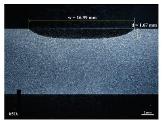
**Fig. 2** — Metallurgical cross-section of laser heat treated D6510 die material.
