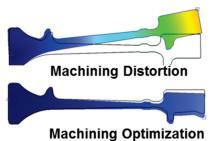
**Fig. 6** — Model predictions of machining distortion for an axisymmetric disk component without prior control of bulk residual stresses (top) and for a disk where prior bulk residual stresses are optimized and specifically controlled. The predicted distortions are magnified to enable visualization and comparison.
