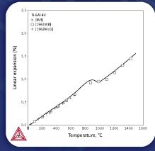
Linear expansion vs Temperature for Ti-6AI-4V
