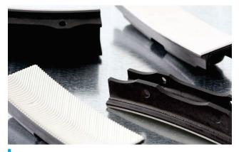
Example of CMC turbine shrouds used on passenger planes and fighter jets. Courtesy of GE Aviation.
