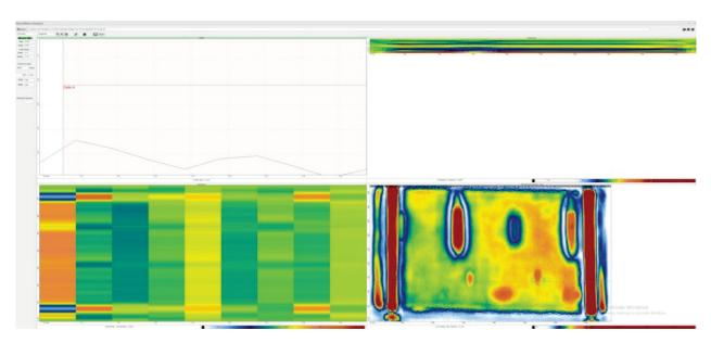
Fig. 5 – Demonstration of MW inspection for defect sizing (depth detection) by using multi-frequency sweeping.
