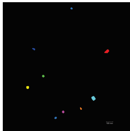
Fig. 4 — Left: One titanium EDS map. Right: The precipitates have been segmented and labeled by Avizo2D.
