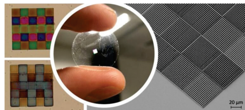
Left, zoomed-in optical microscopy images showing the pixelated sensor in response to different vapors; center, photo of the glass substrate showing the 3D-printed sensor; right, scanning electron microscopy image of the pixelated sensor, showing the different heights of the periodic structure. Courtesy of Trinity College Dublin.
