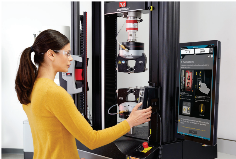
Automated crosshead positioning features ensure the fixture separation is precisely repeated by any technician operating the system.
