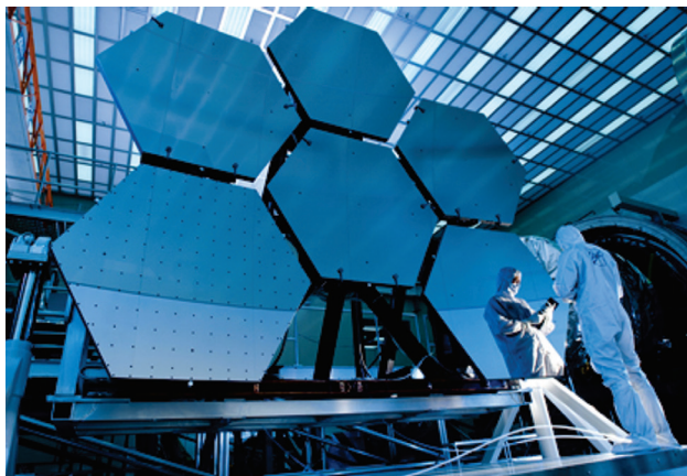
Materion provided 18 hexagonal beryllium mirrors for the James Webb Space Telescope. Courtesy of NASA.
