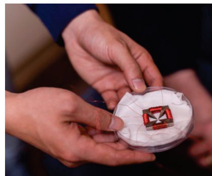
This digital inkjet printer head uses magnetic or dielectric particles.
