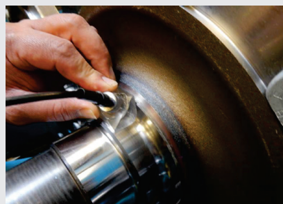
Fig. B — NDT measurement of the case depth in the radius area.
