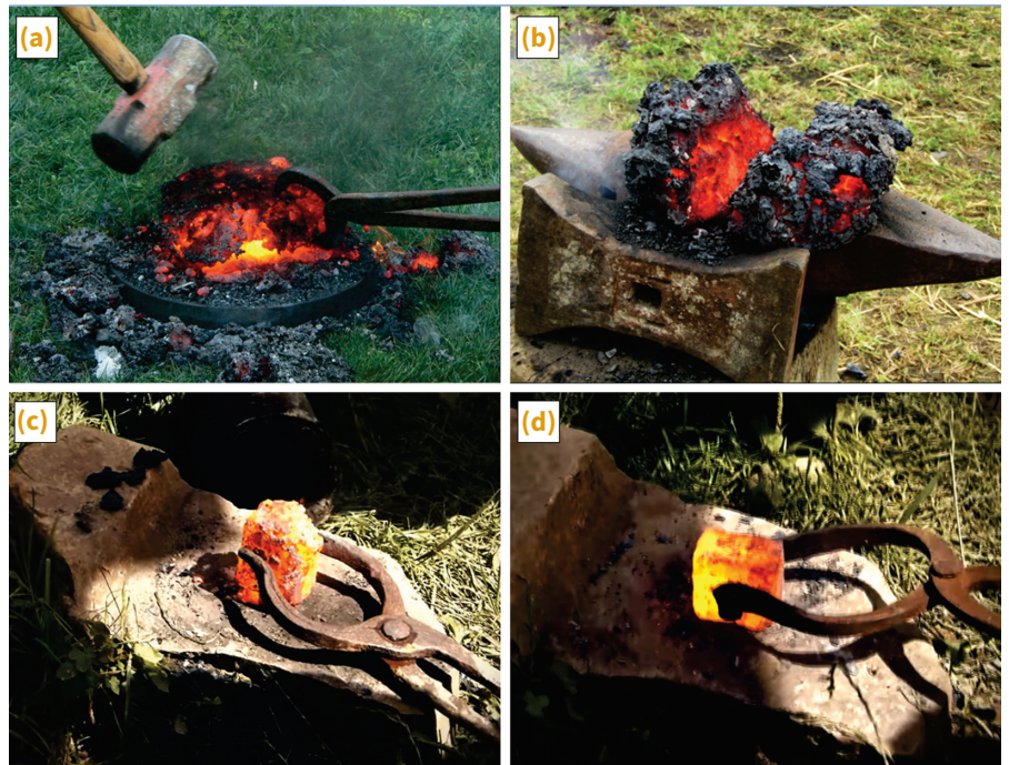
Fig. 2 — Iron bloom processing: (a) slag removal and bloom consolidation, showing pieces of slag surrounding the bloom; (b) a large bloom split using a maul and sledge hammers; (c, d) hammer hand-forging to the required shape. Adapted from various experimental archaeometallurgy sources.
