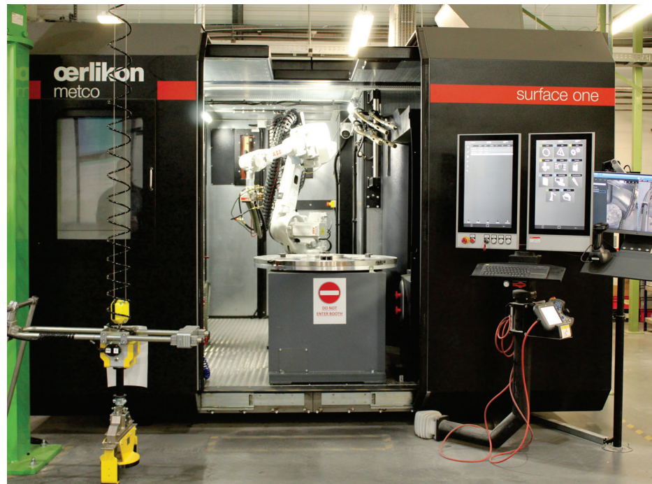
Fig. 1 — Thermal spray cell, encompassing aspects of minimum standards for cleanliness, ergonomics, and layout. Courtesy of Turbine Surface Technologies Ltd.
