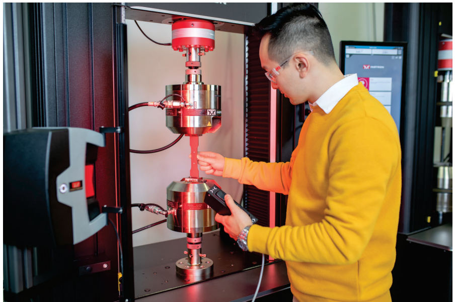
Mechanical testing of an AM coupon using a video extensometer.
