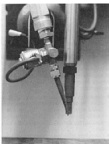
FIG. 16 TYPICAL SETUP USED TO MEASURE WELDABILITY USING THE IMPULSE DECANTING TEST. SOURCE: REF 11
