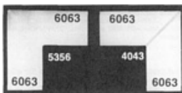
FIG. 7 CLEAR ANODIC COATING ON 6063 WELDS MADE WITH ALUMINUM-MAGNESIUM (5356) AND ALUMINUM-SILICON (4043) FILLERS
