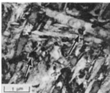
FIG. 11 TRANSMISSION ELECTRON MICROGRAPH OF LASER WELD FUSION ZONE IN RAPIDLY-SOLIDIFIED/POWDER METALLURGY TI-8AL-2.8SN-5.4HF-3.6TA-1Y-0.2SI ALLOY SHOWING YTTRIUM-ENRICHED DISPERSOIDS (INDICATED BY ARROWS) LOCATED ALONG SOLIDIFICATION SUBSTRUCTURE BOUNDARIES. SOURCE: REF 17
