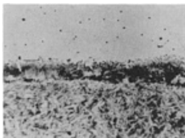
FIG. 2 PHOTOMICROGRAPH SHOWING WELD INTERFACE CROSS SECTION OF 0.81 MM (0.032 IN.) THICK HIGH-CARBON (0.9 WT% C) STEEL ULTRASONICALLY WELDED TO 0.81 MM (0.032 IN.) THICK IRON. 1000×
