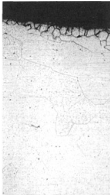
FIG. 14 INTERGRANULAR CORROSION OF THE INSIDE SURFACE HAZ OF E-BRITE STAINLESS STEEL ADJACENT TO THE WELD FUSION LINE. ELECTROLYTICALLY ETCHED WITH 10% OXALIC ACID. 100x. SOURCE: REF 47
