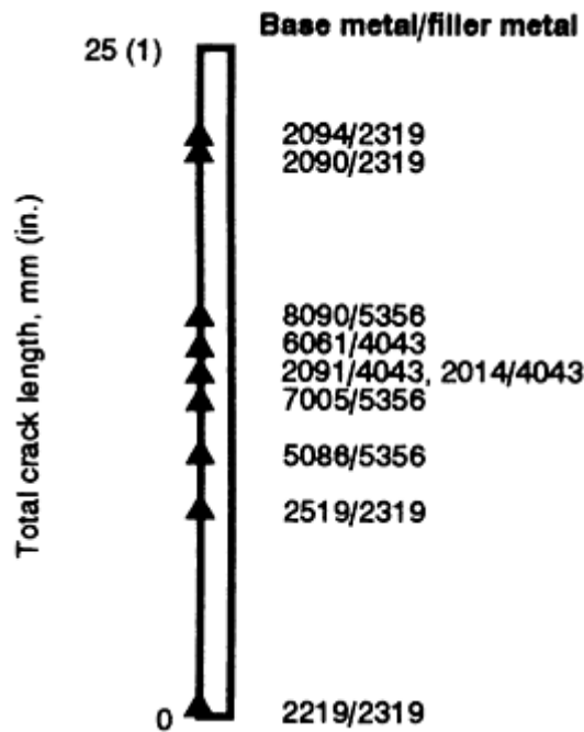
FIG. 3 TRANS-VARESTRAINT WELDABILITY DATA FOR ALUMINUM ALLOYS. SOURCE: REF 25
