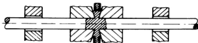
End of second upsetting sequence
