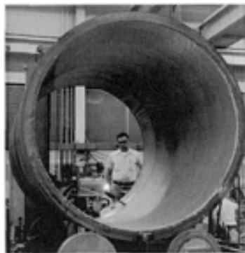
FIG. 29(A) WELD CLADDING OF A 1.8 M (6 FT) INNER DIAMETER PRESSURE VESSEL SHELL WITH 50 MM (2 IN.) WIDE, 0.64 MM (0.025 IN.) THICK STAINLESS STEEL STRIP. COURTESY OF J.J. BARGER, ABB COMBUSTION ENGINEERING
