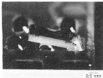
FIG. 12 DRAWBRIDGING OF A LEADLESS CERAMIC CHIP RESISTOR (OPTICAL MACROSCOPY). COURTESY OF SANDIA NATIONAL LABORATORIES
