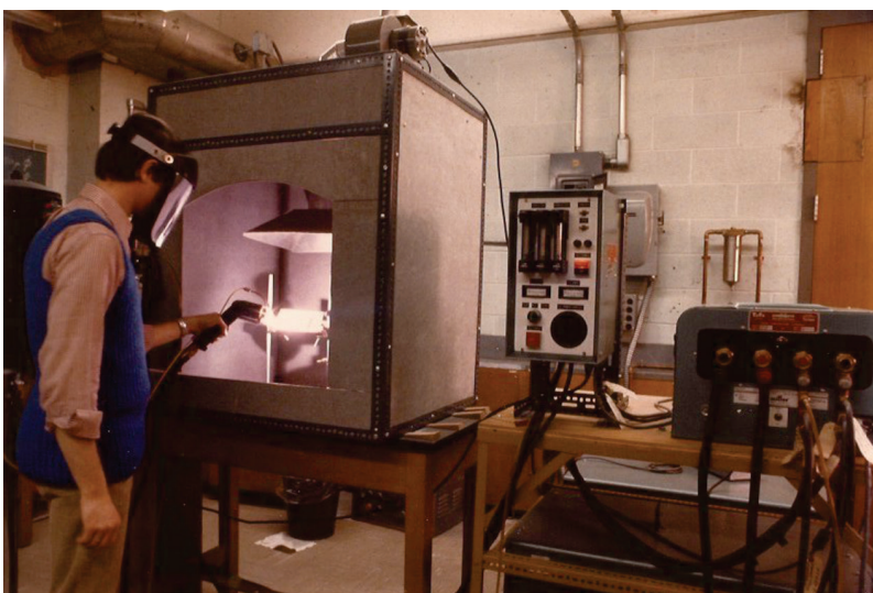
Fig. 1 — A "glove box" plasma spray set-up at Stony Brook used by the late Dr. Volker Wilms in the 1970s.
