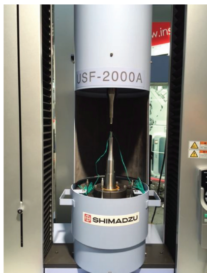
Fig. 4 — External view of the mean stress loading jig.
