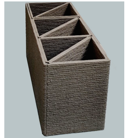
A building envelope prefabricated using 3D printing. Courtesy of Mehdi Chougan.
