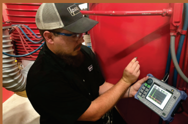
Ipsen vacuum chamber wall thickness testing.
