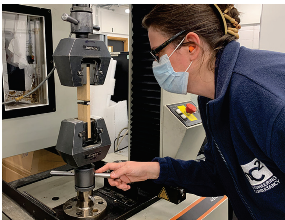
Researcher Nicola Symonds performs a tensile test on a wood sample. Courtesy of NMRN.
