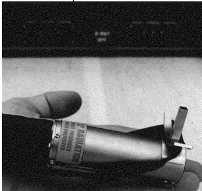
Fig. 14 Photograph of a miniature x-ray diffractometer for the one angle technique arrangement of XRD stress measurement. This device incorporates a Ruud-Barrett position sensitive scintillation detector and is capable of being inserted in a 101.60 mm (4 in.) inside diameter for measuring residual stress (Ref 39).
