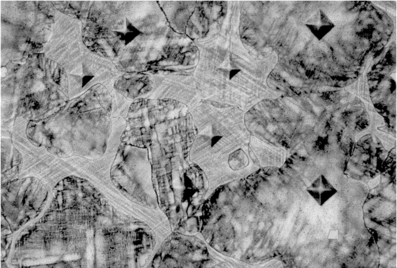
Fig. 25 Vickers indents (100 gf) in the matrix (dark) and in the intergranular beta (white) phase in an age-hardened as-cast beryllium copper (C 82500) that was burnt in solution annealing (differential interference contrast illumination, aqueous 3% ammonium persulfate and 1% ammonium hydroxide). 500×
