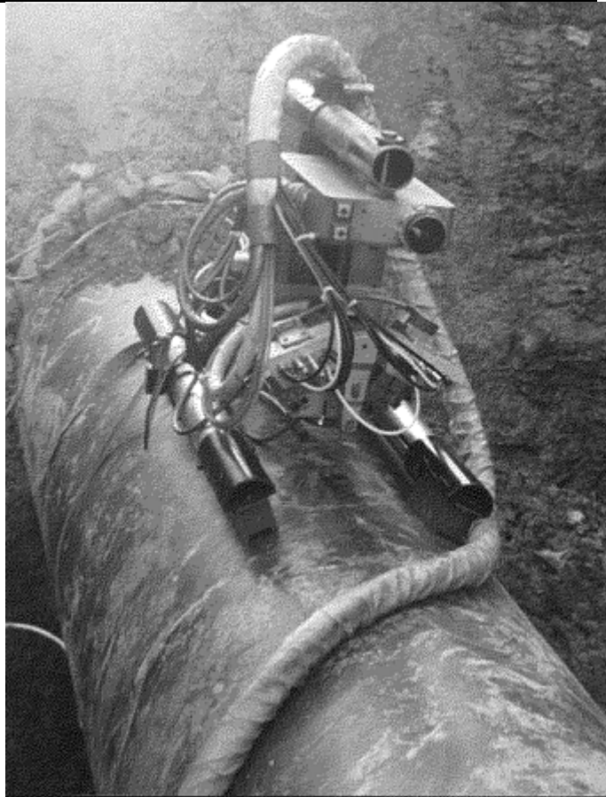
Fig. 1 Measurement of residual stresses on a gas pipeline in the field using a portable x-ray diffraction instrument. (Courtesy of Proto Manufacturing)
