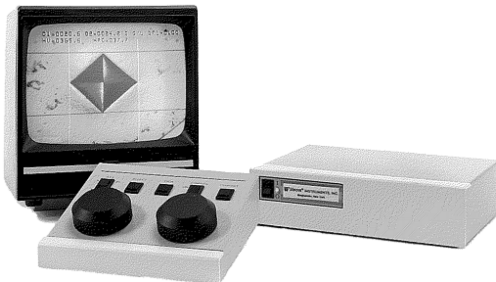
Fig. 23 Vilar system for digital image processing of Vickers indents
