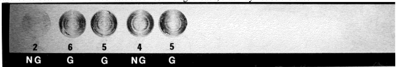
Fig. 8 Sequence of galling tests on block specimens. Source: Ref 17
