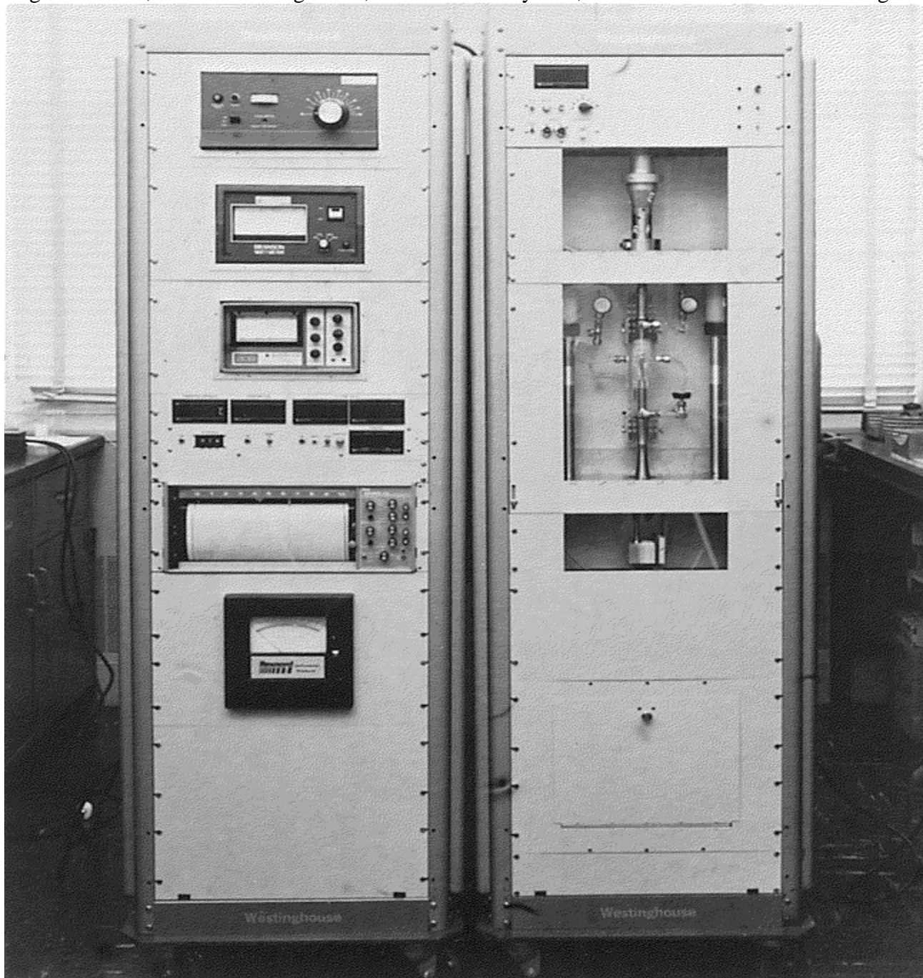
Fig. 4 Portable 20 kHz corrosion-fatigue machine with mean load capability
