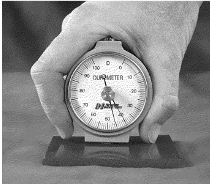
Fig. 9 Handheld durometer for testing hardness of plastic and rubber materials. Courtesy of NewAge Industries
