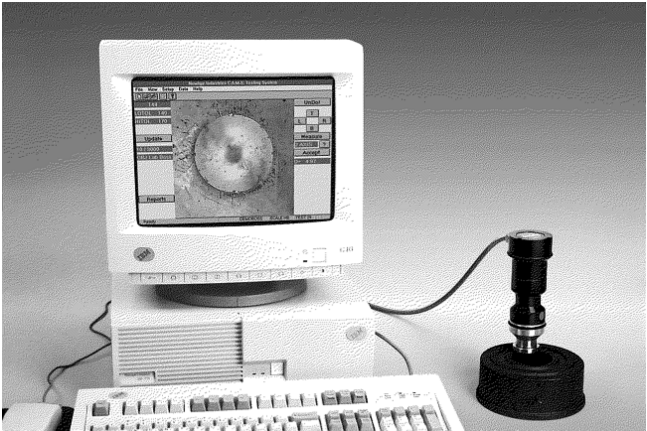
Fig. 14 Computerized Brinell hardness testing optical scanning system
