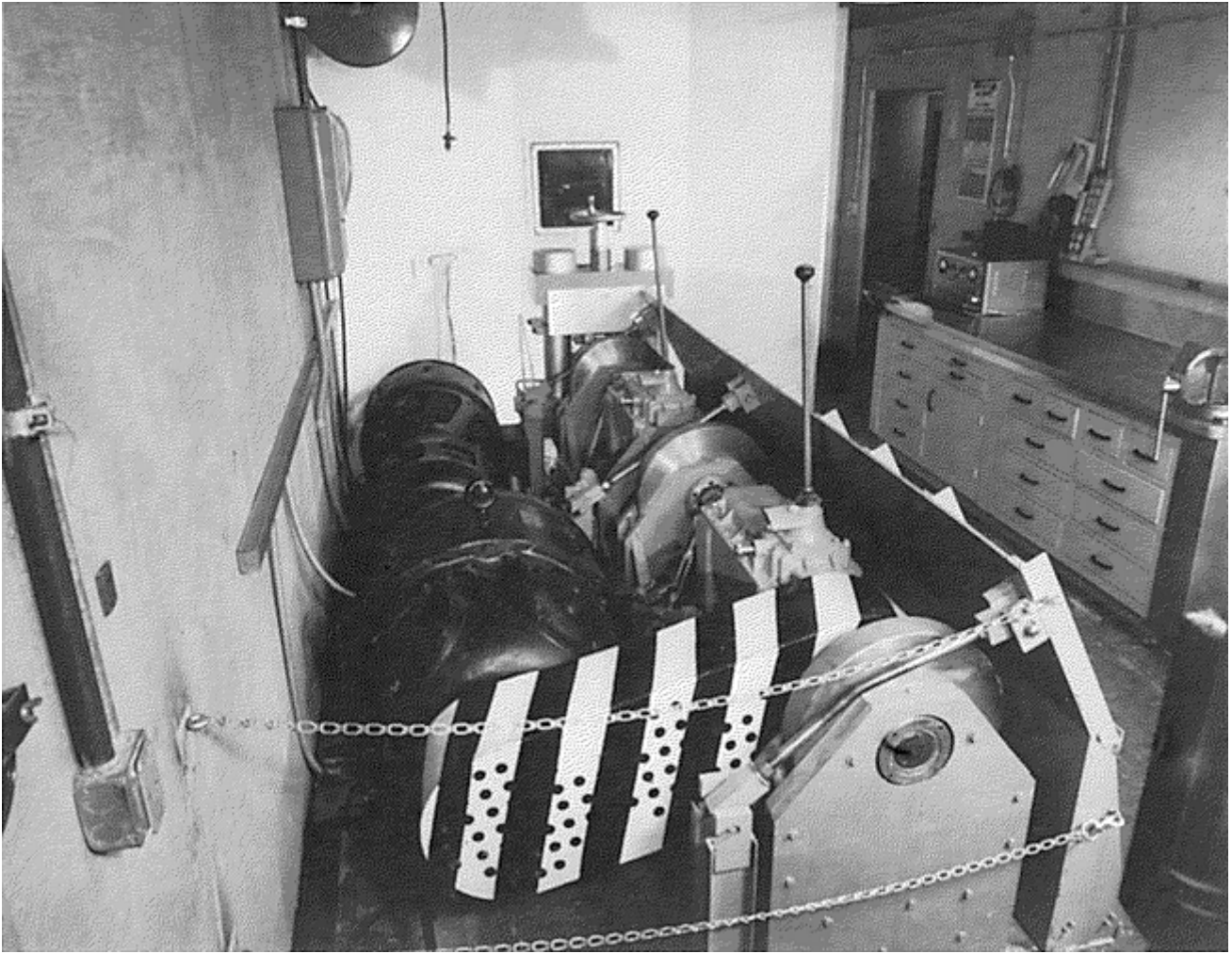
Fig. 2 Typical cam plastometer facility. Direct-current motor and generator are on the left; three flywheels and two transmissions are on the right; two-post loading frame is at rear. Courtesy of Los Alamos National Laboratory
