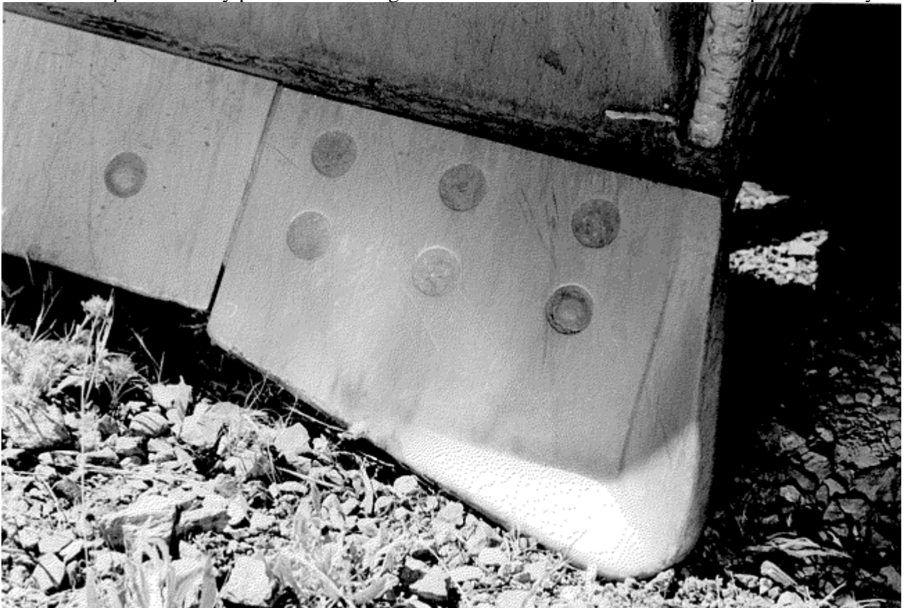
Fig. 1 Extent of abrasion on a bulldozer blade. Notice the width and depth of the wear scars.
