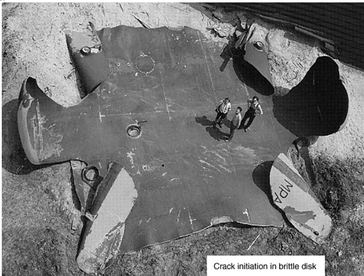
Fig. 20 Catastrophic failure at internal pressure of a feedwater tank
