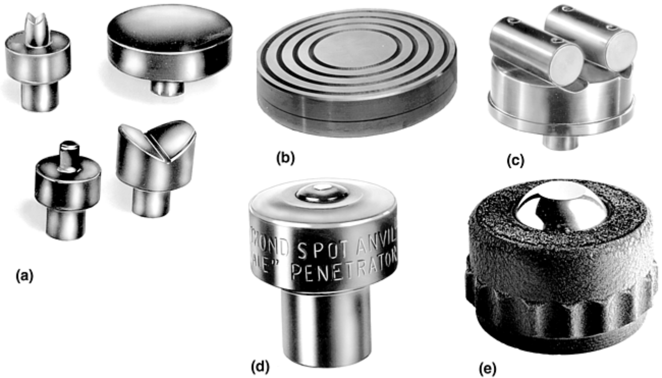
Fig. 7 Typical anvils for Rockwell hardness testing. (a) Standard spot, flat, and V anvils. (b) Testing table for large workpieces. (c) Cylinder anvil. (d) Diamond spot anvil. (e) Eyeball anvil
