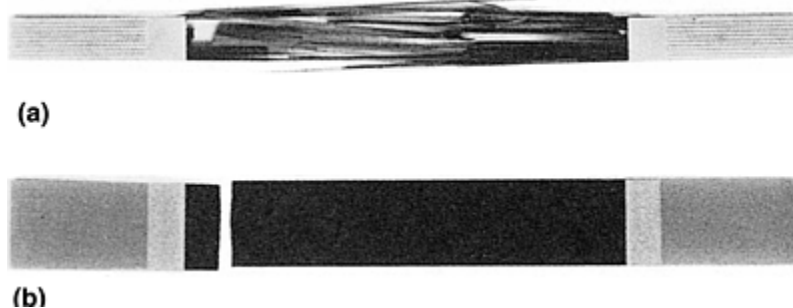
Fig. 6 Commonly observed, acceptable failure modes of (a) 0°, and (b) 90° carbon/epoxy unidirectional composites
