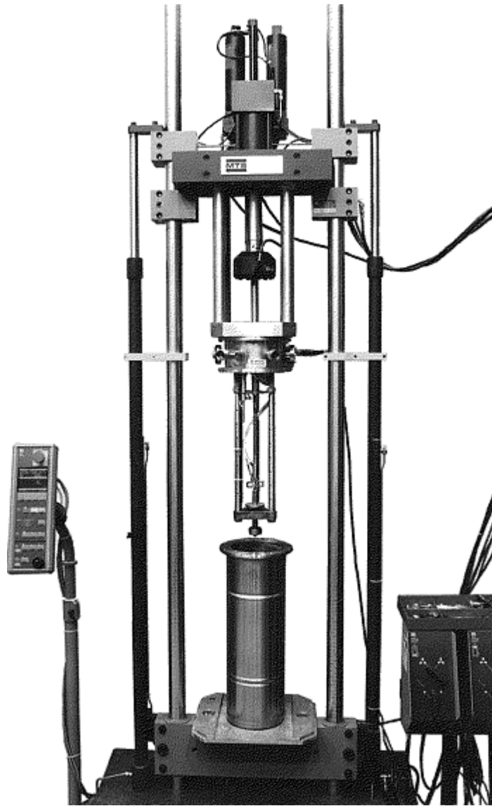
Fig. 2 A 100 kN capacity test machine equipped with cryostat for low-temperature testing
