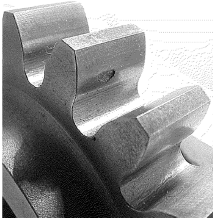
Fig. 4 Specimen gear with arrow-shaped surface origin pit
