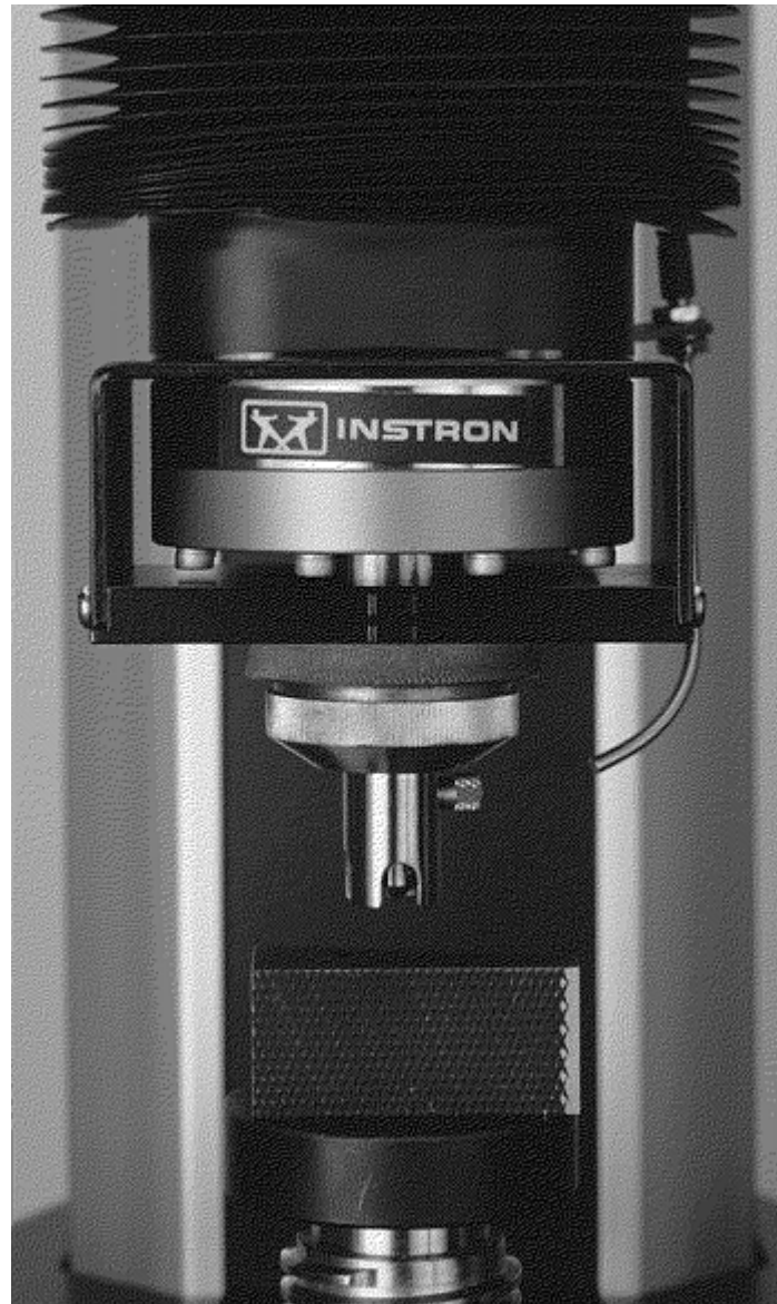
Fig. 8 Rockwell tester with removable clamping assembly
