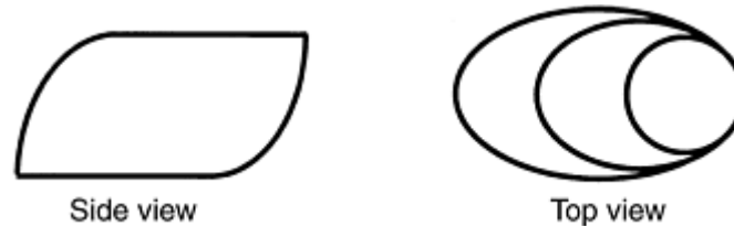
Fig. 5 Schematics of a tilted (sheared) tested specimen
