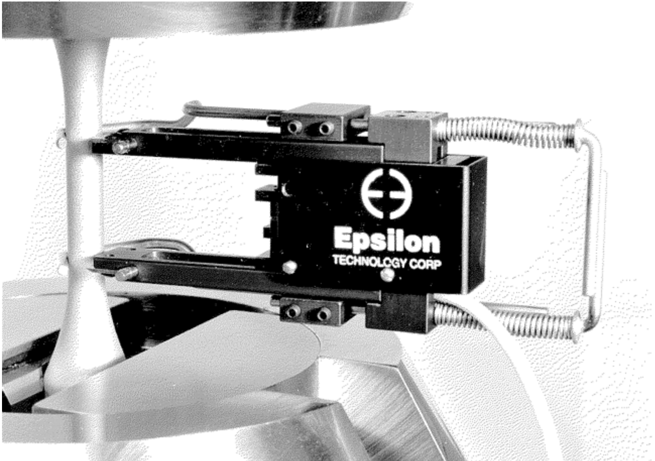
Fig. 10 Test specimen with an extensometer attached to measure specimen deformation. Courtesy of Epsilon Technology Corporation
