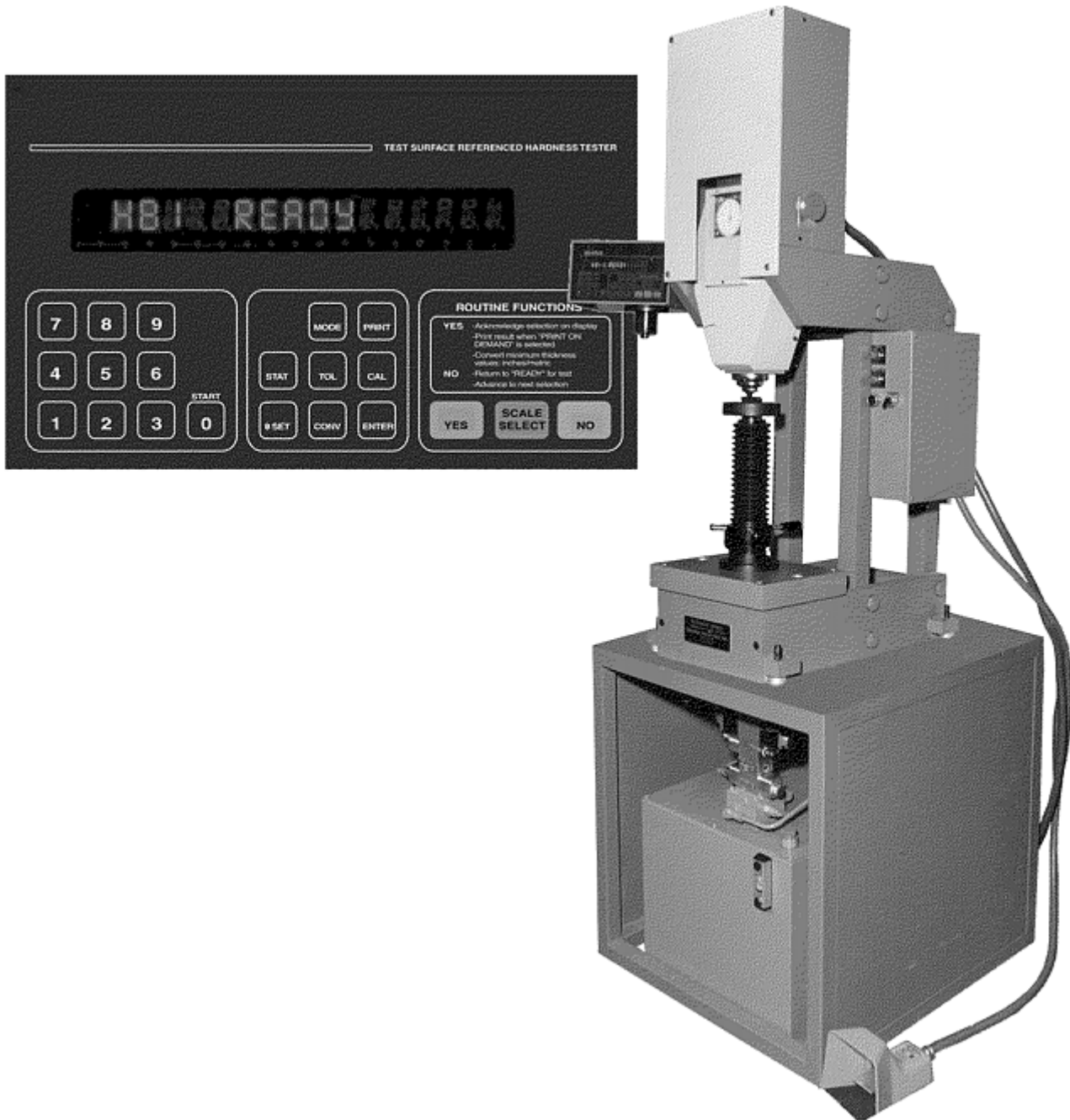
Fig. 17 Automatic Brinell hardness tester with digital readout. Courtesy of NewAge Industries
