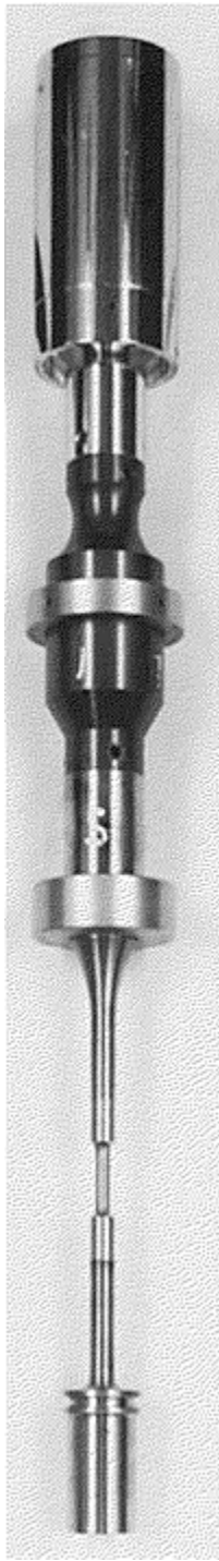
Fig. 6 Typical 20 kHz acoustic wave train
