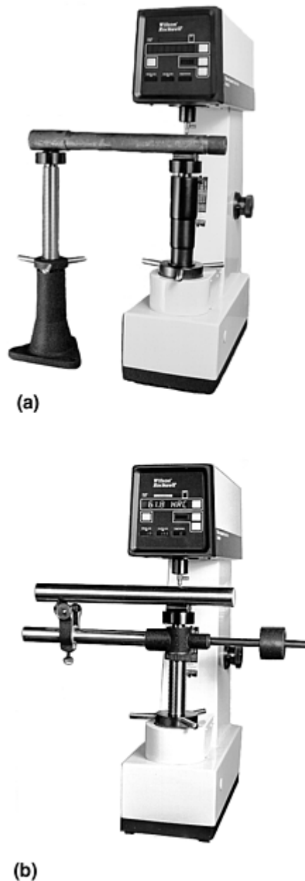
Fig. 9 Rockwell test setups for long testpieces. (a) Jack setup. (b) Variable rest setup
