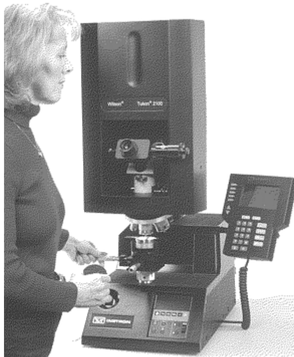
Fig. 5 Closed-loop load-cell microindentation hardness tester
