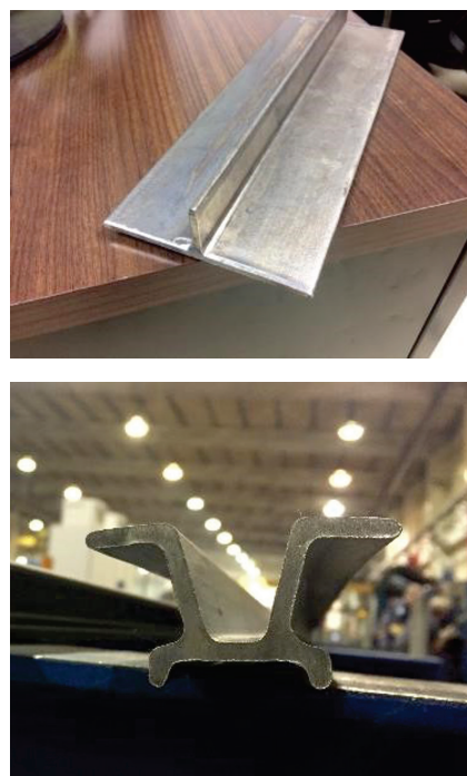
Fig. 4 — Near net extrusions produced in Ti-64. A sample cut from the T-profile (top) and complex geometrical profile (bottom) are beta extruded to over 30 ft long.
