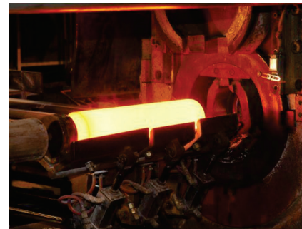
Fig. 1 — Forward extrusion process where the ram pushes the hot metal through the die.
