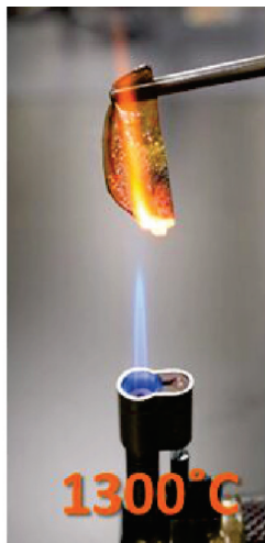
A cellulose-derived film has high thermostability and is flame resistant. Courtesy of JAIST.
