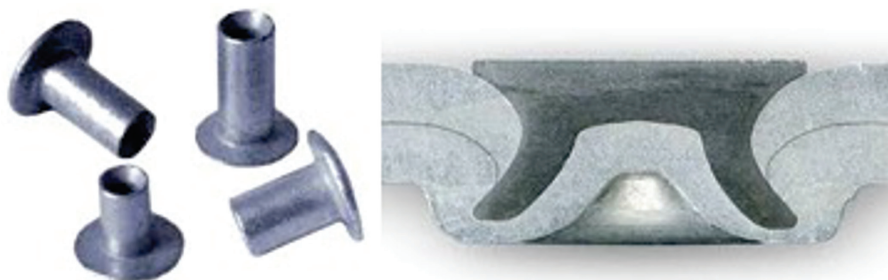
Fig. 1 — From left, self-piercing rivets and typical cross section of a joint. Courtesy of Stanley Engineered Fastening.
