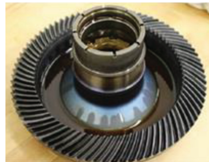
Fig. 2 — Ferrium C64 input shaft (top) and gearshaft (bottom) imaged after 85 minutes of loss-of-lubrication testing in Bell Helicopter's Future Advanced Rotorcraft Drive System program. Results show minor scuffing on the gear teeth but no signs of surface damage or failure. Courtesy of Bell.
