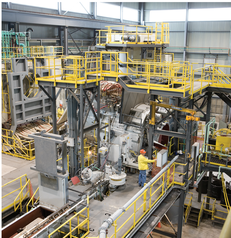
Carpenter Technology's 22 metric ton vacuum induction melter where Ferrium C64 is manufactured. Courtesy of Carpenter.
