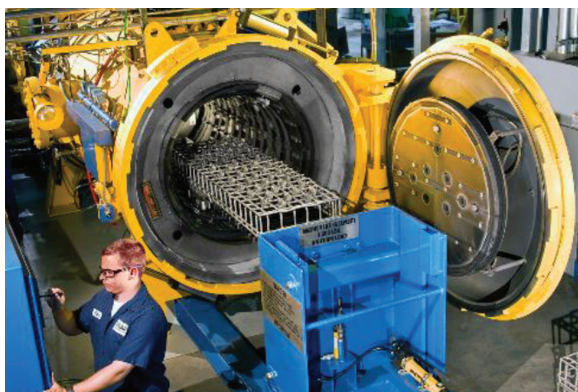
Rack of gears undergoing vacuum heat treatment at Solar Atmosphere's Souderton, Pa., facility. Courtesy of Solar.
