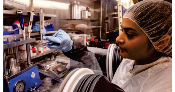
Doctoral student Jyotshna Pokharel assembles a lithium-ion battery in which lithium metal is used in place of graphite as the anode material. Courtesy SDSU.
