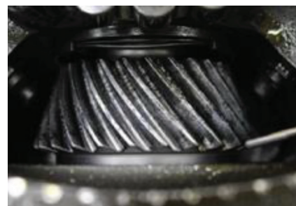
Ferrium C64 steel FZG type test gear chemically processed by REM Chemical in as-ground (top of image) and after isotropic superfinishing (bottom). REM can achieve Ra ranges in 1-6 \mu\text{m} for C64. Courtesy of REM.
