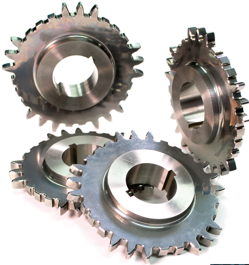
Fig. 3 — Single tooth bending fatigue gears made of Ferrium C64, processed via additive manufacturing on an EOS M 290 machine, heat treated and superfinished.
