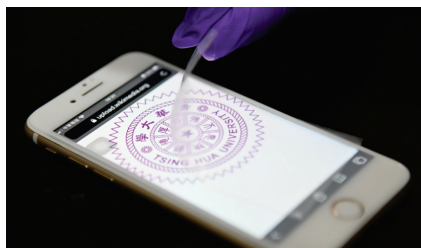
Mobile phone featuring a self-sanitizing cover produced from a material made by extracting chitin from squid bones. Courtesy of NTHU MSE, Taiwan.
